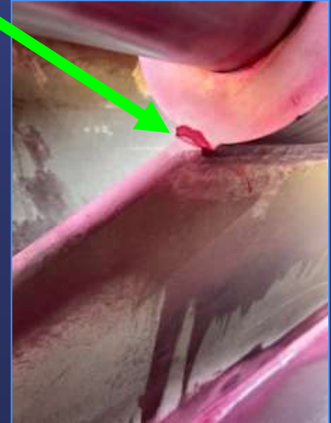
Liquid penetrant testing on valve body
