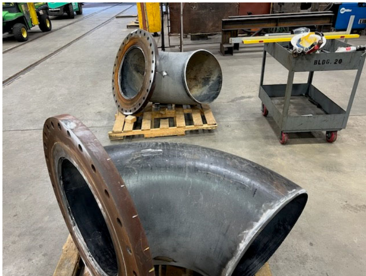
The La Verne Shops fabricated reducing elbows (left) and leg support (right) for a 24-inch bypass line at OC-88 on the AMP
