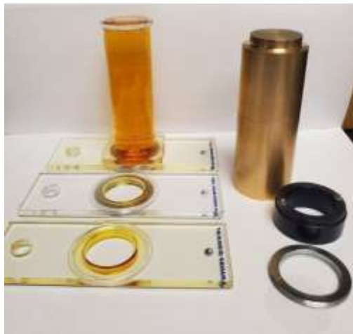
Hydrobios chamber, tool, and glass retainer (left) and hydrobios chamber under microscope (right)
