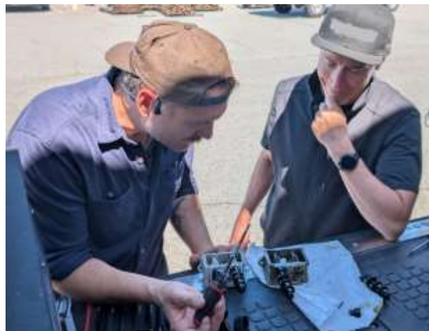
Diemer plant staff participating in testing limit switch on actuator
