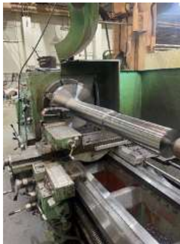
3D Model of shaft (left), machining of shaft (middle), and fit test of shaft and lift nut (right)
