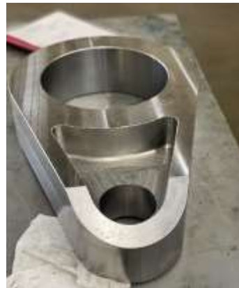
3D model of the lifter lever (left) and completed lifter lever (right)
