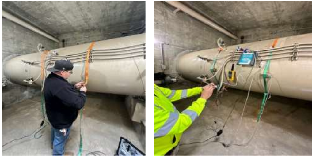
Staff installing “clamp-on” flowmeter (left) and verifying flow measurements (right)
