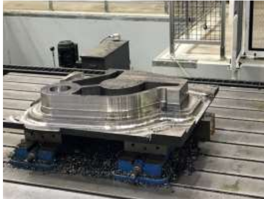
3D Models of rotating assembly (left) and lift nut (middle), and machined lift nut (right)
