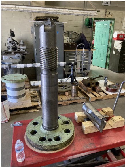
Broken discharge valve plug shaft
