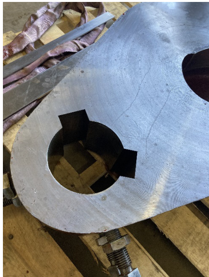
Fractured rotator (left), machining new rotator (center), and test fit of new lift nut to new plug shaft (right)
