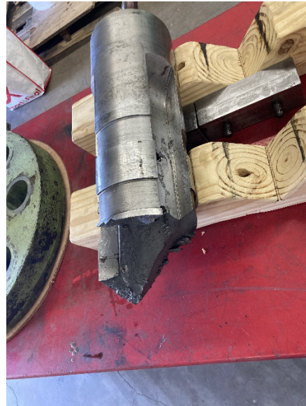
Broken discharge valve plug shaft
