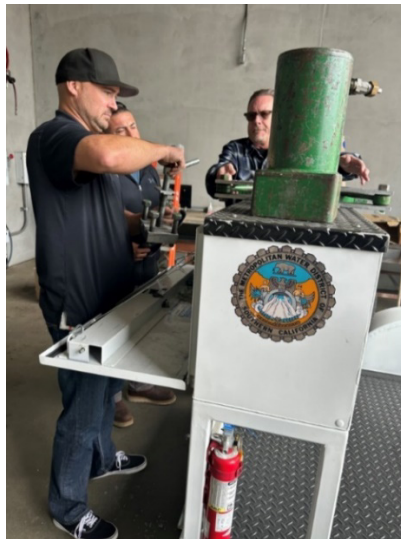
Staff inspecting C-Kit to stop a simulated chlorine leak (left) and installing C-Kit with LACFD observing (right)
