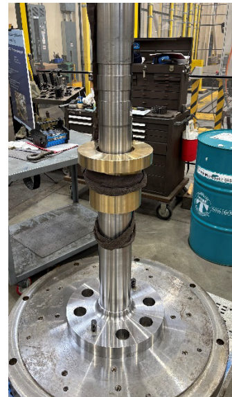
Fractured rotator (left), machining new rotator (center), and test fit of new lift nut to new plug shaft (right)
