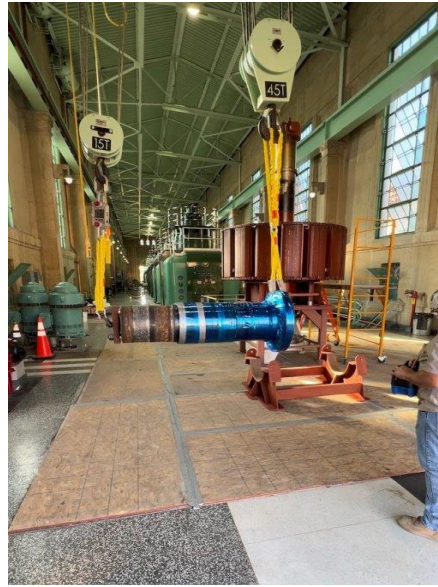
Staff fabricating a new pump shaft cradle at Eagle Mountain pumping plant
