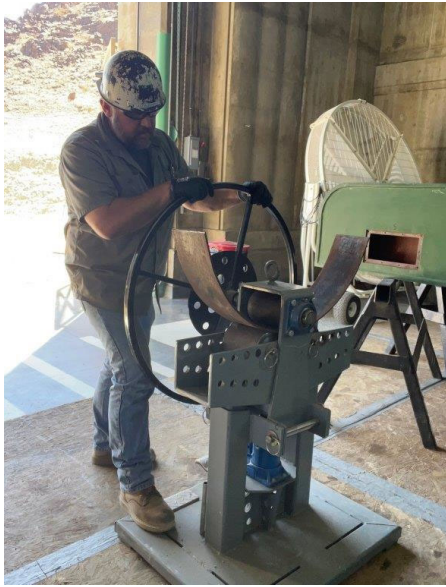
Staff fabricating a new pump shaft cradle at Eagle Mountain pumping plant
