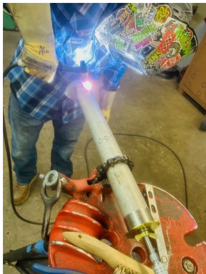
Staff fabricating new stainless pipe manifolds for CRA pump cooling water systems
