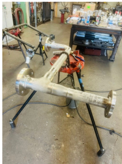
Staff fabricating new stainless pipe manifolds for CRA pump cooling water systems
