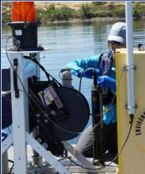
Maintenance on a source water monitoring platform
