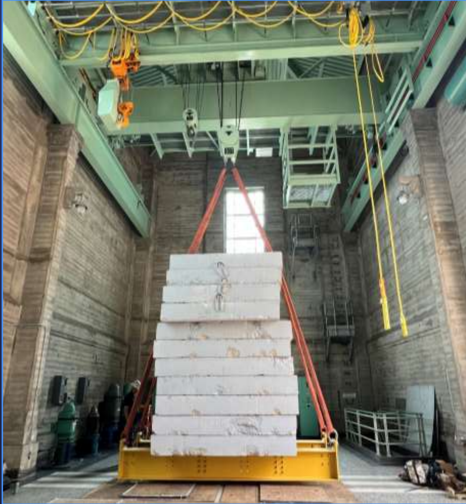
Load testing of overhead crane at Intake Pumping Plant
