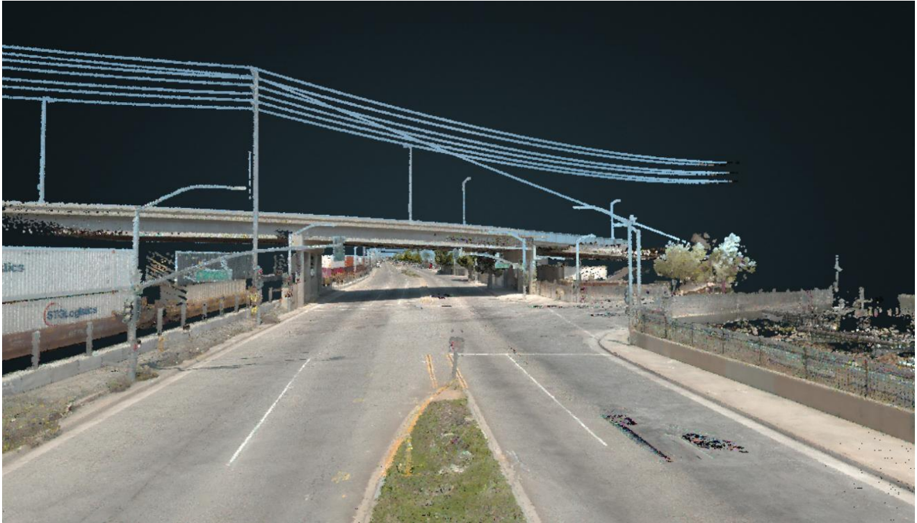
PWSC Reaches 1 and 2—Point cloud data from LiDAR survey
