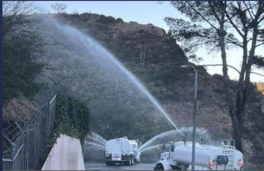
Wetted facility perimeter for fire protection
