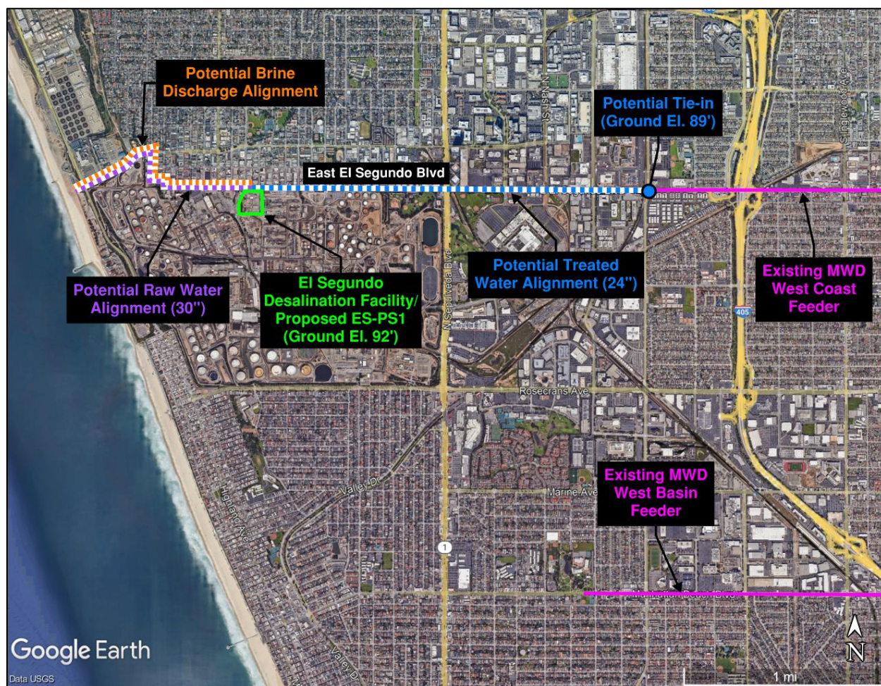
Figure 7.5 El Segundo Seawater Desalination Facility Potential Alignment
