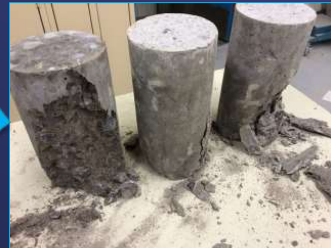
Concrete Cylinder Compressive Strength Testing
