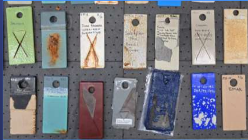
Failed Coating Test Coupons
