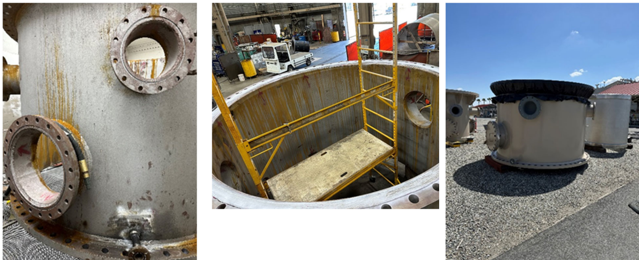
As-found condition (left), weld build-up (middle) and completed refurbishment (right) for a component of the DVL sleeve valve
