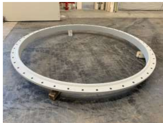
Carbon steel follower after fabrication (left) and finished coating (right) for the Upper Feeder pipeline
