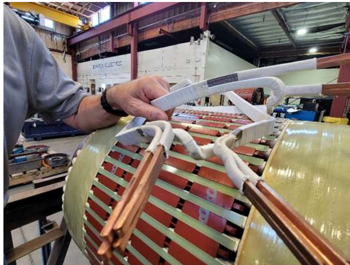
Staff inspecting a CRA motor armature coil prior to vendor installation
