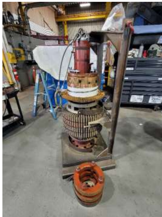
An armature at a local motor shop before machining for the CRA
