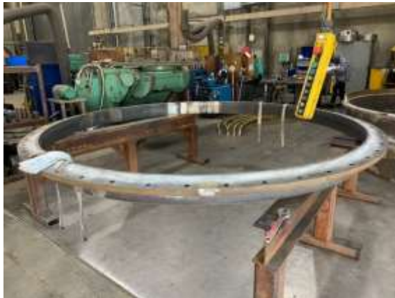
Carbon steel follower after fabrication (left) and finished coating (right) for the Upper Feeder pipeline
