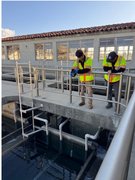
Staff collecting water quality samples (left) and analyzing samples for chlorine residual (right) at the Weymouth plant
