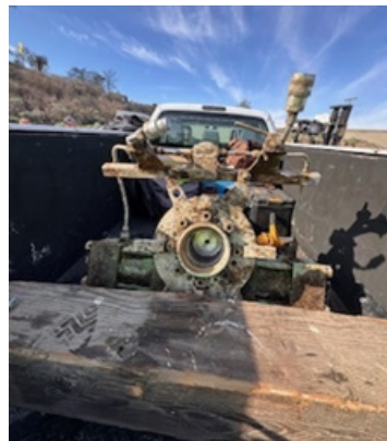
Existing actuator after pressure washing (left) and removed actuator for refurbishment (right)
