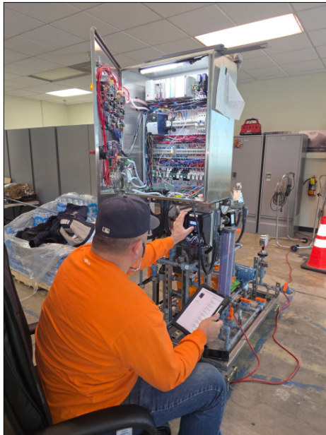
Staff programming a variable frequency drive (left) and completed piping and instrumentation (right) for a chemical feed pump skid
