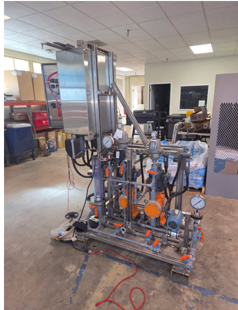
Staff programming a variable frequency drive (left) and completed piping and instrumentation (right) for a chemical feed pump skid
