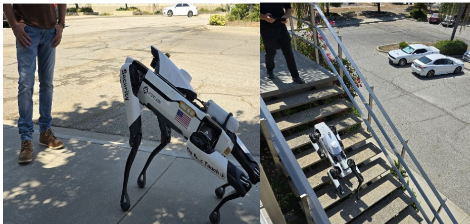
Securitas is piloting a robotic patrol dog at Jensen WTP as part of potential new contract guard service option
